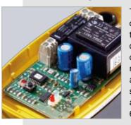
The control electronics operate the discharge valve with such precision that all collected condensate is discharged without any loss of compressed air. This not only maximises compressed air use but also leads to considerable energy savings. All electrical components are protected from water ingress (IP 65, ECO DRAIN 30/31: IP54).
