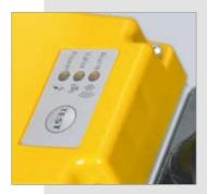
Should an alarm situation occur (e.g. a blocked discharge line), the unit waits 60 seconds before switching to alarm mode which then allows operation on a timer basis. A flashing LED indicates the alarm and a volt-free contact enables alarm signals to be sent to a control centre or compressor controller (from ECO DRAIN 31).
